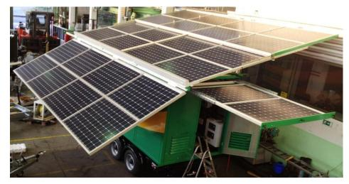
KUNZ has designed and assembled Mobile Solar Power System which draws 9,234 W solar powers first and followed by 43,68 kWh lead-acid batteries and finally relying on 53 kW back-up diesel genarators power as the final fallback for the power.
