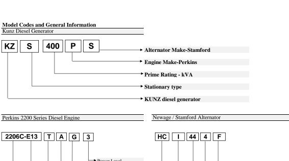
► Power Level Genset engine Air to air charge cooled Turbocharged Electronic 13 liters 2200 Series, 6 cylinder
