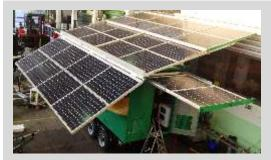
PV Modules KUNZ's PV modules are European origin and they are as unique as like the whole design. 28 panels are suppliying over 9 kW.
